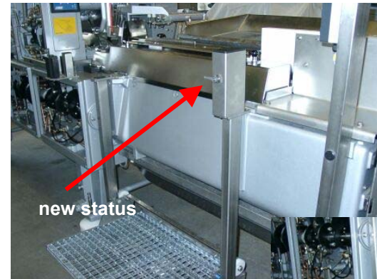
It is also possible to lift up the operator platform for better cleaning
