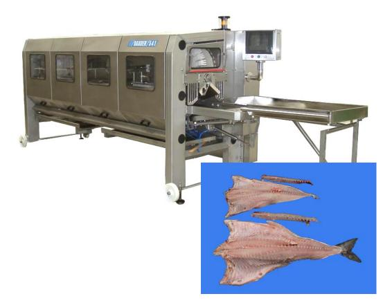
perfect saltfish cut whole working range without adjustment high flexibility regarding the cuts high capacity - high yield less downgrades, due to electronic measurement and movement of the tools automatic neckblood-removal device available easy to clean
